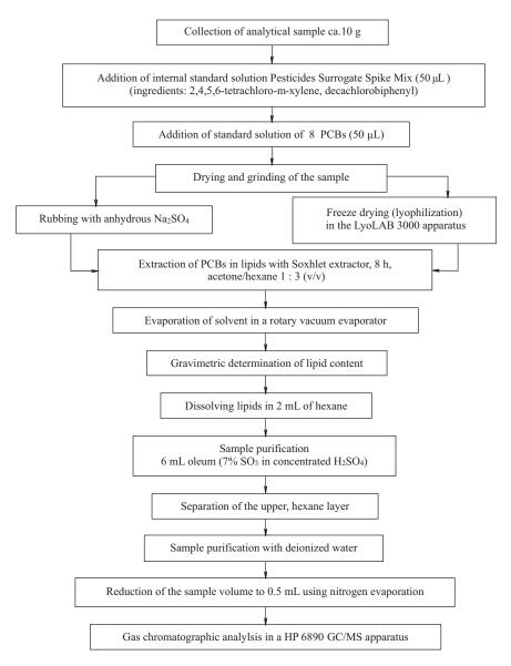
Fig. 2. The flowchart of PCB analysis in fish samples
