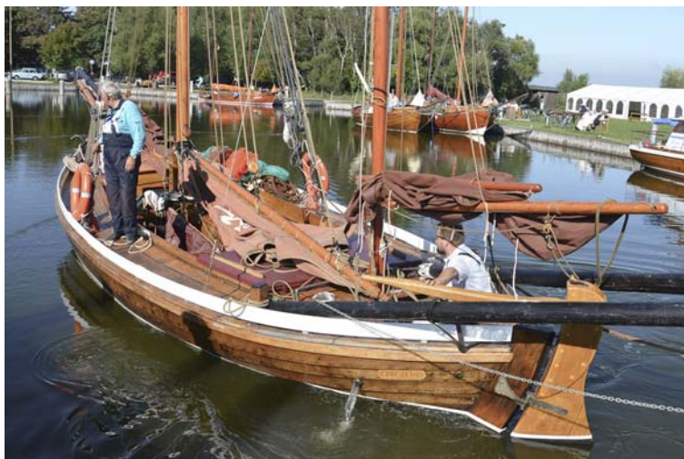
Fig. 17. A fully equipped Zeesboot departing for a trip (NE Germany); Note black Zeesbäume (a single Zeesbaum parallel to the bowsprit and two other on the stern); nets ready to be deployed on the bow (starboard) (Photo by Martin Rurik, http://zeesbootfahrten.de )
